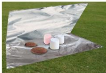
SOLAR OVEN: fold the foil-covered card in half to form the oven base and lid.
